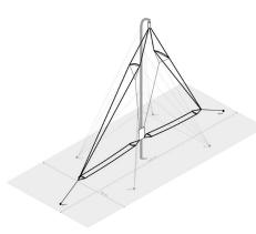
The Delta antenna is a high performance, omni-directional, broadband antenna that is suited to base-to-base or base-to-mobile communication over short to medium distances.
