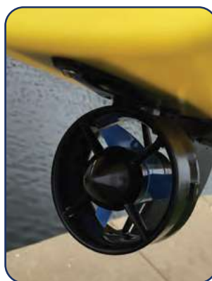
Powerful differential thrusters for maneuverability
