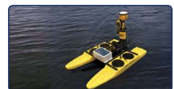
HyDrone™ ASV with Trimble SPS 585 and TSC3
