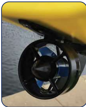
Powerful differential thrusters for maneuverability
