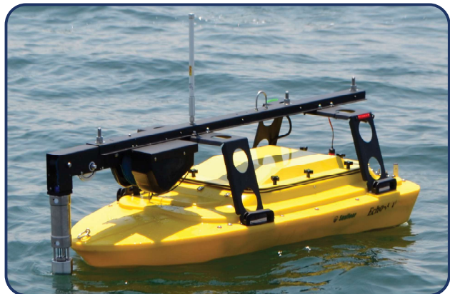
Valeport SWiFT SVP mounted on QuickCast System
