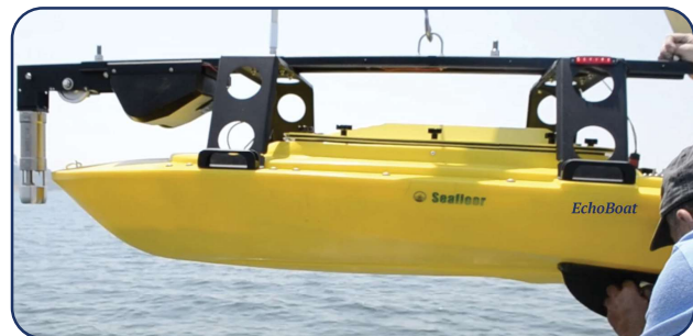
QuickCast Winch with Valeport SWiFT SVP mounted on EchoBoat USV
