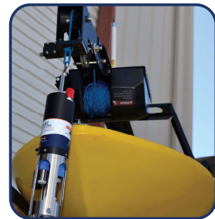
Winch comes spooled with 30m of rope
