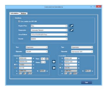
Within the Utilities section, one will be able to handle the Geodetic Calculator, a basic tool for transforming coordinates. With more than 70 countries and 1,200 available datums, it remains one of the most versatile calculators in the market.
