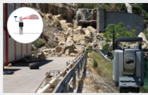
This kind of monitoring is based on the combination of various diverse positioning sensors such as Total Stations and/or GNSS with additional sensors that can supply complementary data and information for the topographical study (thermometers, inclinometers, electro-accelerometers etc.).
