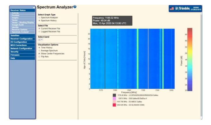
In this example the DME transmitters are not causing any major problems to L5 tracking, however, this may not always be the case where frequencies are closer to the GNSS
