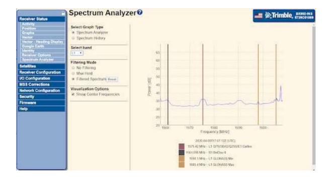
Three different selections are available to filter the data. With No Filtering mode, the spectrum analyzer passes the raw data sampled directly to the display. This is useful for attempting to catch transient type signals such as radars.
