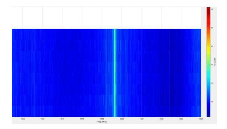
The onboard spectrum analyzer can help speed up this task significantly. In the following example poor positioning performance from a vehicle navigation system prompted a closer look at the signal tracking and Spectrum Analyzer.
