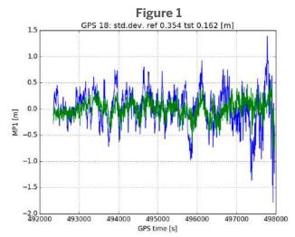
Evaluating all GPS satellites from the same data set in a roof top environment yields an average multipath reduction of 31% with the new technique (Figure 2).
